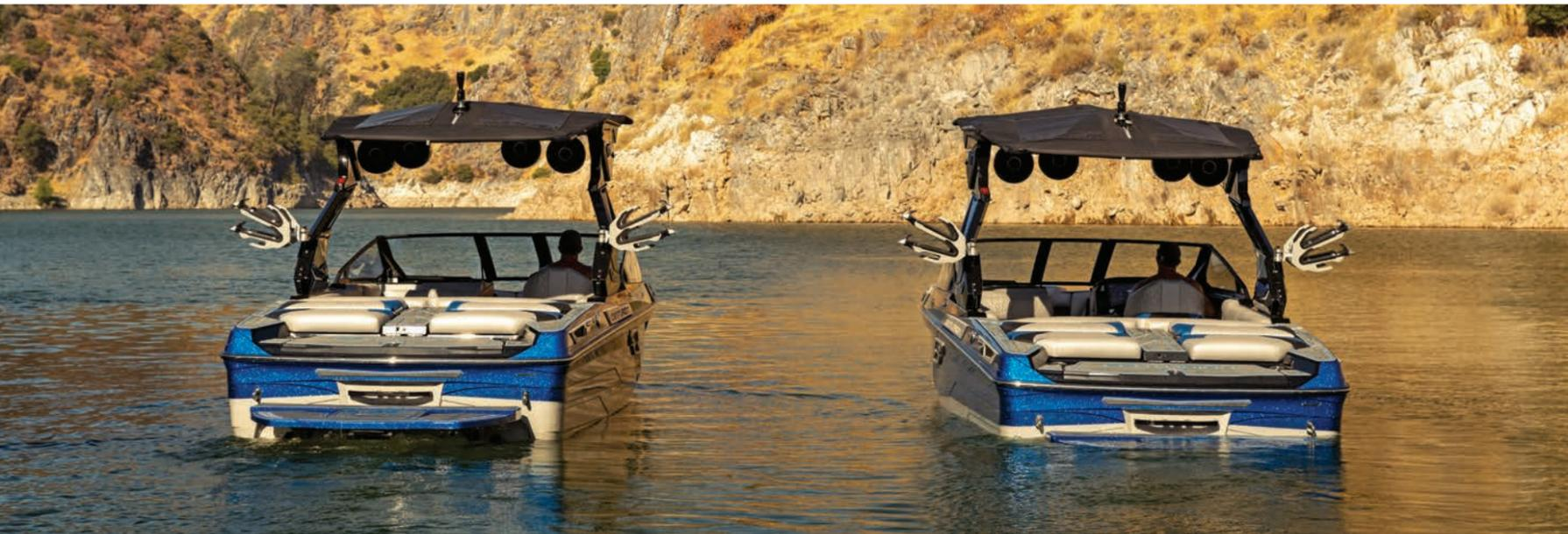
**ABOVE:** As much as 5850 pounds of ballast displaces the hull 10 inches farther into the water to generate the waves and wakes Centurion is known for. There is no replacement for displacement.
