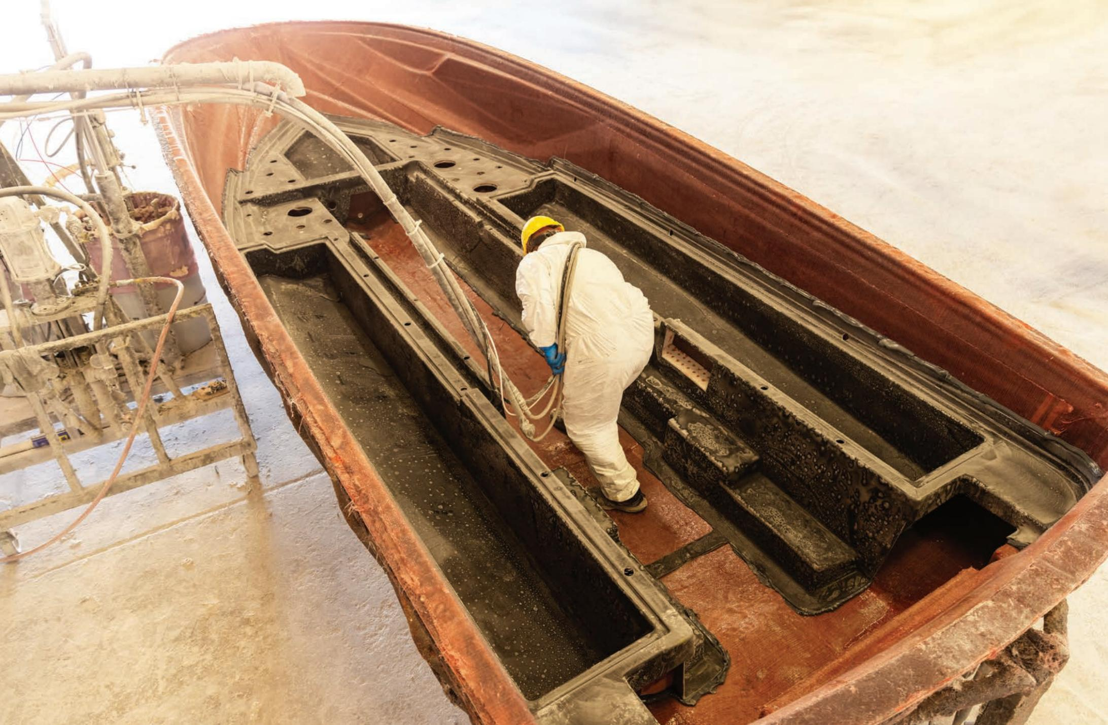
**LEFT:** A Centurion has strength at its core with a specifically designed stringer system that houses as much as 3350 pounds of ballast and welcomes six stable mounting points for a PCM engine.
