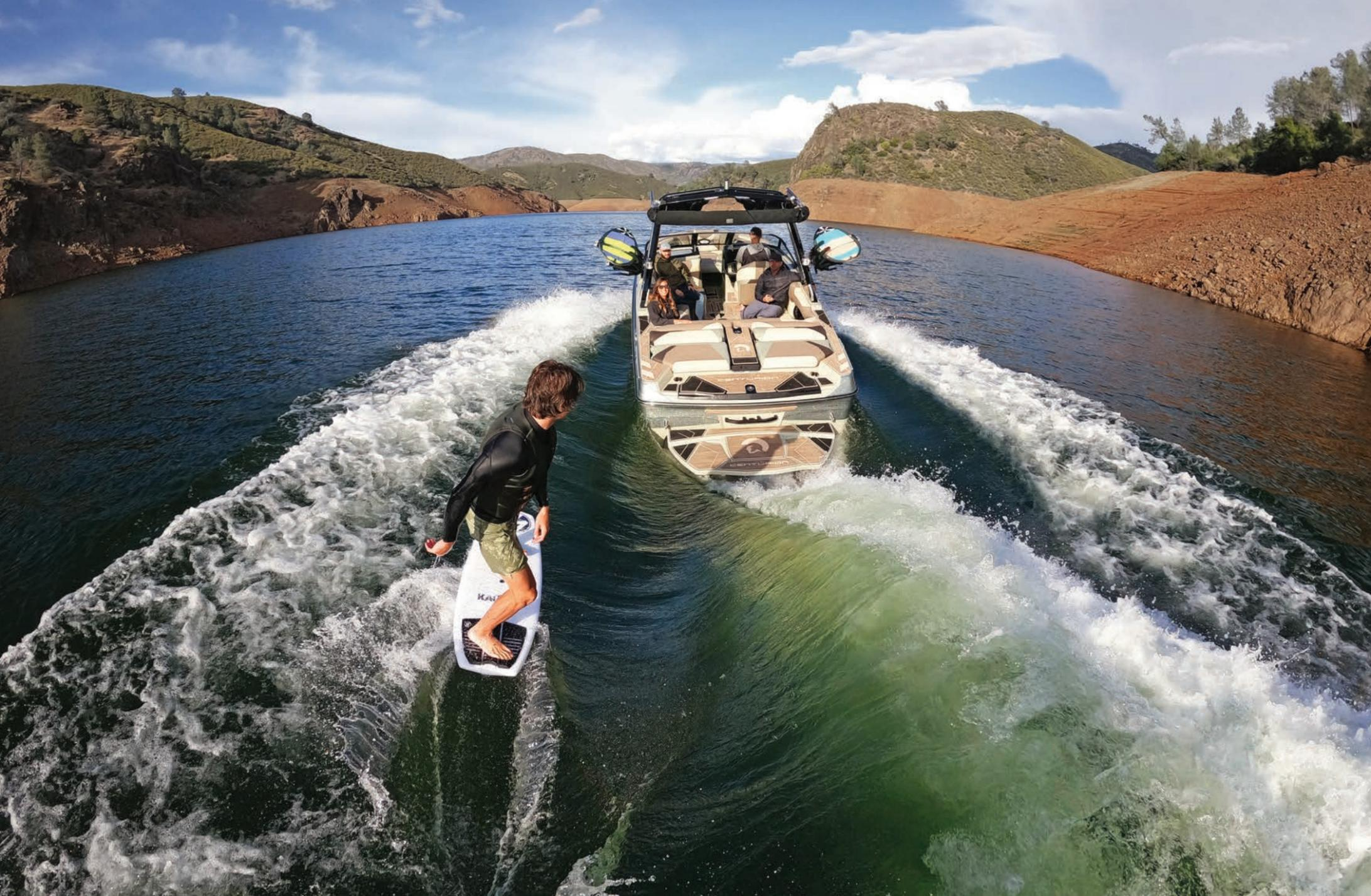
**LEFT:** Ballast and passenger weight can be evenly distributed in a Centurion to achieve a professional level surf wave with the help of QuickSurf Pro. QSP creates lift opposite the surf side to displace the surf-side corner slightly more and create the curl.
