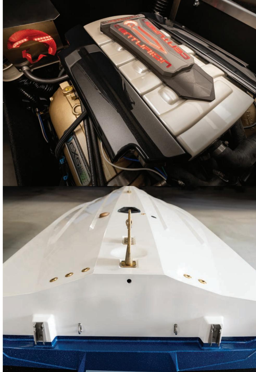
**LEFT TOP:** The supercharged direct injected ZZ8S from PCM offers 665 foot pounds of torque with a Power Plus Super Duty Transmission and a 1.7:1 gear reduction. This golden lit Centurion engine option looks as good as it performs even fueled by 89 octane.
