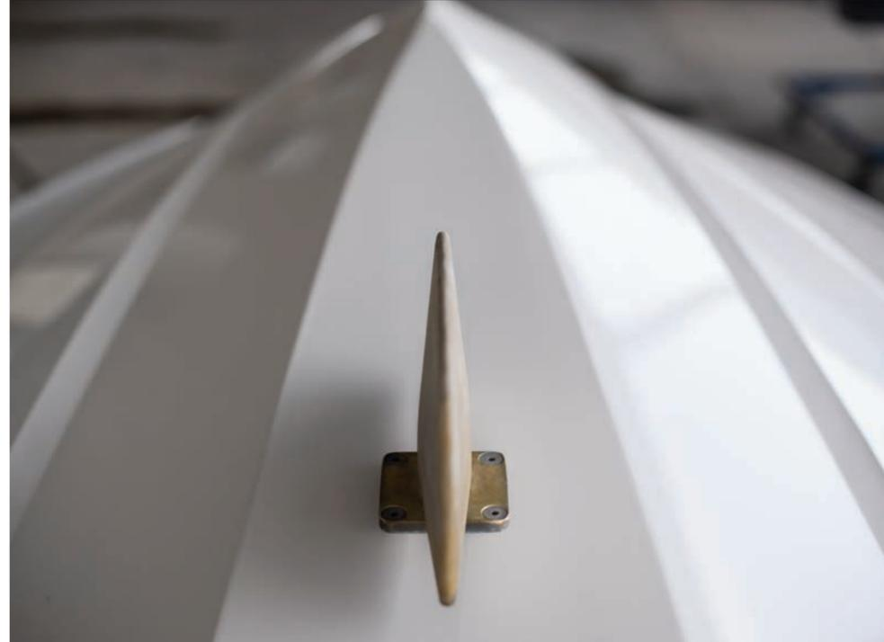
**LEFT TOP:** This is a Centurion Ri hull mold between color sprays during the Gel Coat process.
