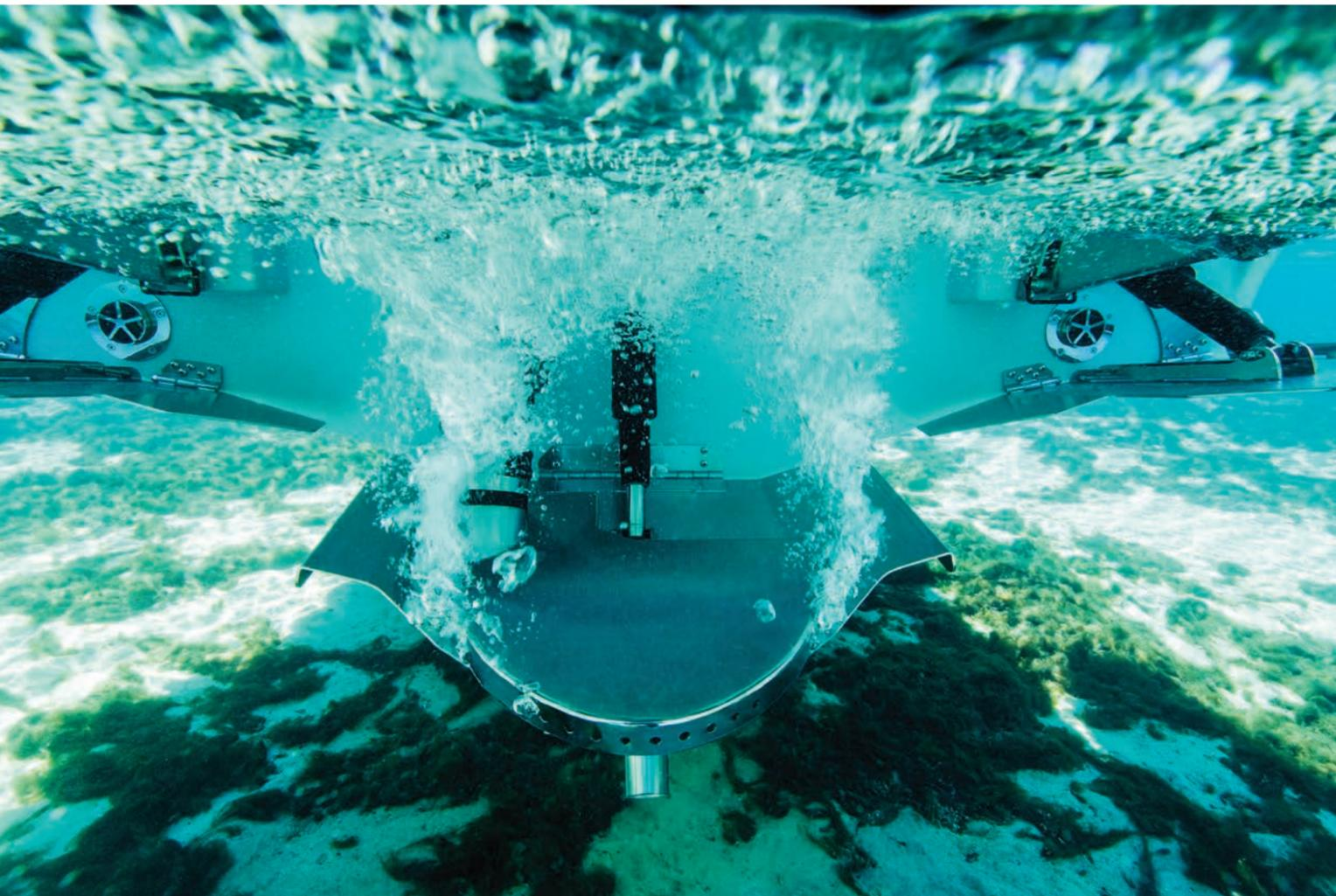
**LEFT:** The Silent Stinger Wake Plate is a trim tab that adjusts your attitude. Not only does it change the running attitude of a Centurion, it also changes your attitude on the water by keeping the engine noise inside voice quiet.
