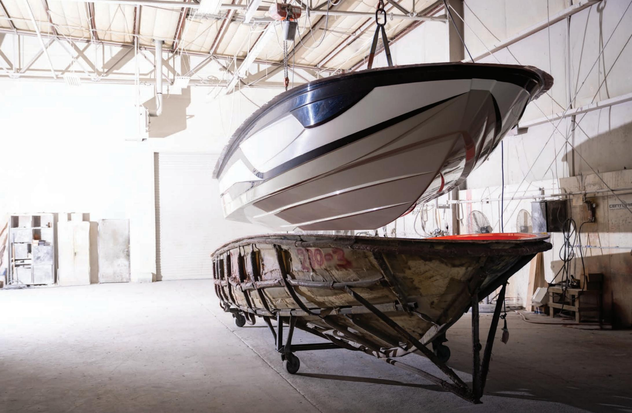
**LEFT:** This 2025 Centurion Ri230 is being pulled from the mold, in the Pull and Grind Department at the Merced, California factory.
